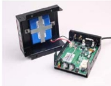
Internal battery connection.
