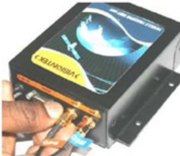
GSM & GPS antenna connection.
